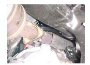
**4.** Starting at the top, to remove the driver's side manifold first remove the driverside heat shield on the manifold. Then remove the manifold hardware through the top of the engine compartment.
