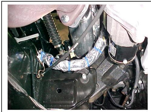
3. NOW STARTING ON PASSENGER SIDE, REMOVE HEAT SHIELD AND MANIFOLD FOR INSTALLATION OF GIBSON LOG HEADER. CLEAN HEAD SURFACE OF ANY DEBRIS BEFORE INSTALLATION.
