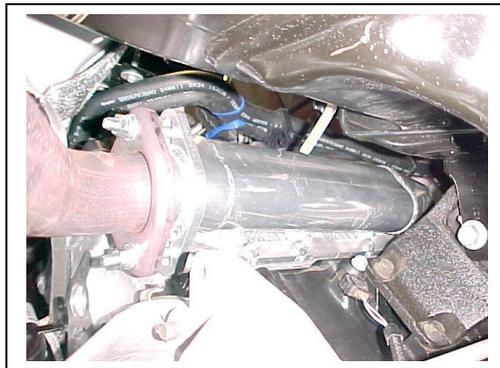
6. NOW CONNECT BATTERY CABLE BACK-UP AND CHECK FOR LEAKS. AFTER WARM UP LET ENGINE COOL DOWN AND TORQUE HEADERS ONE MORE TIME TO PREVENT LEAKS. THEN AFTER 200 TO 300 MILES RE-TORQUE HEADERS AGAIN. THEN WE RECOMMEND DOING THIS AT EVERY OIL CHANGE. THIS WILL ENSURE GIBSON HEADERS TO LAST TO THEIR FULLEST POTENTIAL.
