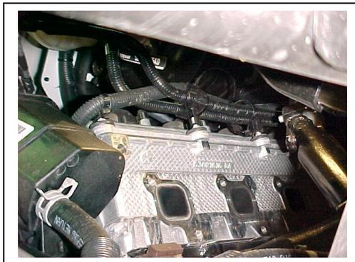
4. NOW NOTICE ON THE PASSENGER SIDE THAT YOUR TWO HEATER HOSES ARE CLOSE TO THE MANIFOLD. USE SUPPLIED Z-TIES TO TIE HEATER HOSES OUT OF THE WAY FROM THE LOG HEADER TO HELP PREVENT HEAT DAMAGE TO HOSES.
