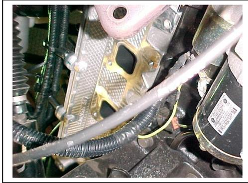
2. NOW ON DRIVERSIDE INSTALL GIBSON LOG HEADER AND SUPPLIED GASKET, HARDWARE TORQUEING TO 30 TO 35 FTLBS. AFTER LOG HEADER IS INSTALLED NOW INSTALL STARTER BACK INTO TRANSMISSION. NOW USING SUPPLIED HEADER-WRAP AND Z-TIES WRAP STARTER WIRES TO PROTECT THEM FROM ENGINE HEAT, AS SHOWN IN PICTURE!
