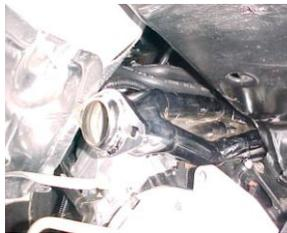
INSTALL SUPPLIED EXHAUST GASKET AND BOLTS ON THE FOUR BOTTOM HOLES ONLY, LEAVING AT LEAST 3/8" OF A GAP FOR INSTALLATION OF GIBSON HEADER. NOW INSTALL GIBSON HEADER AND THE REST OF HARDWARE TORQUING TO 30 TO 35 FT. OF TORQUE.
