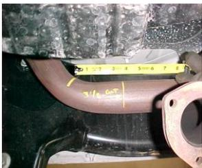
NOW STARTING ON PASS. SIDE FOR REMOVAL OF PASS. SIDE HEADPIPE. YOU WILL NEED TO MEASURE 3 1/2" INCHES FROM CENTER OF BEND AND CUT WITH A HACKSAW OR SAWZALL SHOWN ON PICTURE. MAKE SURE TO DEBURR INSIDE OF REMAINING STOCK HEADPIPE.
