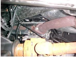
STARTING WITH THE REMOVAL OF STOCK MANIFOLD. REMOVE POSITIVE BATTERY CABLE IN THE ENGINE COMPARTMENT. NOW STARTING WITH THE DRIVERSIDE, REMOVE HEADPIPE AND THEN REMOVE STARTER. FOR EASIER REMOVAL OF STOCK MANIFOLD AND INSTALLATION OF GIBSON HEADERS NOW REMOVE STOCK MANIFOLD AND HARDWARE MAKING SURE TO CLEAN HEAD SURFACE OF ANY DEBRIS, BEFORE INSTALLATION OF GIBSON HEADER.
