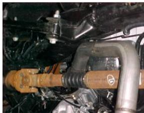
NOW INSTALL PASS. SIDE HEADPIPE ON VEHICLE. NOTICE NOT TO TIGHTEN HARDWARE JUST YET. NOW WITH DR. SIDE INSTALL GIBSON HEADPIPE AND SUPPLIED GASKET USING STOCK FLANGE, MOUNT HARDWARE. BEFORE TIGHTENING HARDWARE CHECK FOR PROPER CLEARANCE. NOW INSTALL SUPPLIED 2 1/4" CLAMP ONTO PASS. SIDE HEADPIPE AND TORQUE DR. SIDE & PASS. SIDE HEADPIPE TO 30 TO 30 FT.
