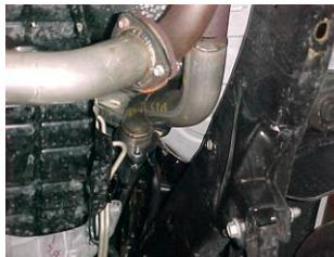
NOW INSTALL SUPPLIED HEAT-WRAP ON PASSANGER SIDE HEATER HOSES ABOVE HEADER USING HEAT WRAP AND WIRE TIES. THIS WILL HELP PREVENT HEATER HOSES FROM MELTING. MAKE SURE TO DOUBLE CHECK THAT ALL FASTENERS ARE TIGHT AND HEATER HOSES ARE PROTECTED BEFORE STARTING UP YOU VEHICAL.
