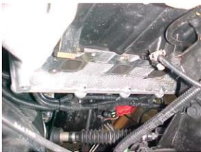
INSTALL DR. SIDE GASKET WITH FOUR BOTTOM BOLTS AND WASHERS LEAVING AT LEAST 3/8" OF A GAP FROM CYLINDER HEAD FOR EASY INSTALLATION OF HEADER. NOW INSTALL GIBSON HEADER AND REMAINING HARDWARE TORQUING FASTENER TO 30 TO 35 FT. OF TORQUE. NOW INSTALL STARTER ON VEHICLE.
