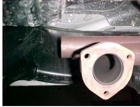
NOW AFTER PASS. SIDE HEADPIPE IS REMOVED. START REMOVING SHIELD, MANIFOLD, AND ALL STOCK HARDWARE. AFTER MANIFOLD IS REMOVED CLEAN HEAD SURFACE OF ANY DEBRIS ON CYLINDER HEAD. FOR EASIER INSTALLATION OF GIBSON HEADER.
