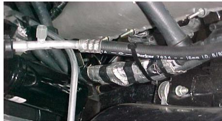
10. Reconnect the exhaust system to the header using the hardware provided.
