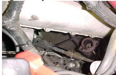
5. Using a scraper, remove all carbon deposits and high spots from head surface. Apply a high temperature gasket sealer to exhaust pipe flare in order to avoid problems due to lack of space later in the installation.
