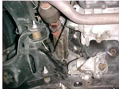
4. To remove the driver's side manifold. First remove the starter. Remove the driver's side manifold, studs and heat shields from the engine, through the top.
