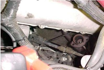
5. Using a scraper, remove all carbon deposits and high spots from head surface. Apply a high temperature gasket sealer to exhaust pipe flare in order to avoid problems due to lack of space later in the installation.
