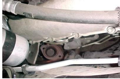
8. Using a scraper, remove all carbon deposits on head surface. At this time apply a high temperature sealer (O2 sensor safe) to exhaust pipe flare in order to avoid problems due to lack of space later on in the installation.
