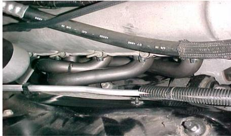
11. Check to make sure there is adequate clearance on battery cables, wire looms, brake lines, etc.
