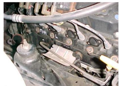
6. INSTALL SUPPLIED PASSENGER SIDE HEADER, GASKET AND SUPPLIED HARDWARE. TORQUE THE HEADER BOLTS TO 30-35 FTS. INSTALL THE 1/4" BOLT, LOCK WASHER AND NUT ONTO THE BRACKET FOR THE DIP STICK. MOUNT THE DIP STICK TUBE TO HEADER USING THE BRACKET. INSTALL SUPPLIED HEAT WRAP ONTO SPARK PLUG WIRE #10 FOR HEAT PROTECTION.
