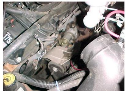
5. ON THE PASSENGER SIDE DISCONNECT THE DIP STICK FROM THE MANIFOLD, BUT DO NOT REMOVE IT. REMOVE THE MANIFOLD, SHIELD AND HARDWARE. CLEAN THE HEAD SURFACE WITH A WIRE BRUSH.
