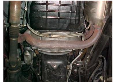
2. STARTING FROM THE BOTTOM LOOSEN THE BOLTS THAT HOLD THE Y-PIPE UP ON THE DRIVERS SIDE AND PASSENGER SIDE FOR REMOVAL OF THE MANIFOLDS.
