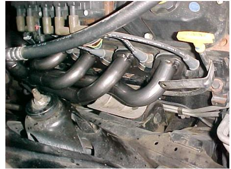
7. RE-INSTALL Y-PIPE WITH SUPPLIED HARDWARE AND TORQUE TO 30-35 FTS. CHECK ALL CONNECTIONS MAKING SURE THEY ARE ALL TIGHT. RE-INSTALL POSITIVE BATTERY CABLE.
