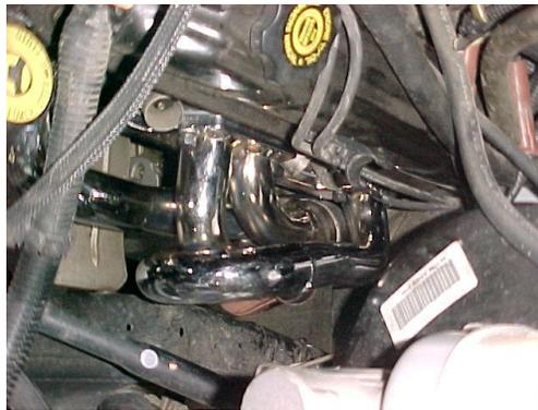
7. For '92-'95 models only begin on the passenger side by removing the EGR tube to the exhaust manifold. Once the bolts have been removed; slightly loosen the tube at the EGR valve (located on the back of the intake manifold) DO NOT REMOVE TUBE.
