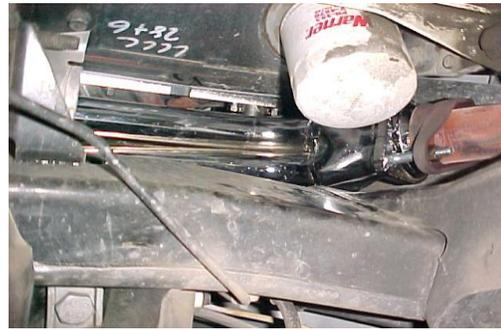
13. Check to make sure there is adequate clearance on plug wires, battery cables, wire looms, brake lines, etc.
