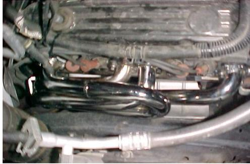
11. Now re-attach air tube to the header using the hardware provided, for vehicles that are EGR equipped. Then apply High Temperature sealer to the base fitting of the EGR valve and re-tighten the air tube.
