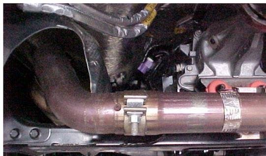
5. DISCONNECT ALL O2 SENSORS. THEN FROM UNDERNEATH THE VEHICLE, LOOSEN THE BOLTS CONNECTING THE Y-PIPE ASSEMBLY TO THE EXHAUST MANIFOLD. (ON 4X4 MODELS, DISCONNECT THE FRONT DRIVESHAFT BY REMOVING THE 4 BOLTS ON THE FLANGE, AND LET THE DRIVESHAFT HANG OUT OF THE WAY.)
