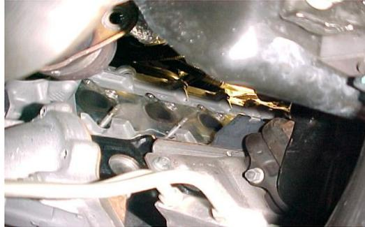
10. USING A SCRAPER REMOVE ALL CARBON DEPOSITS AND HIGH SPOTS FROM HEAD SURFACE, USE CARE NOT TO GOUGE THE ALUMINUM HEADS.
