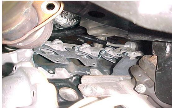
15. ONCE ALL BOLTS ARE SNUG. LOWER MOTOR BACK DOWN AND RE-TORQUE ENGINE MOUNT. TORQUE DOWN BOLTS STARTING WITH THE CENTER BOLTS FIRST. RECOMMENDED TORQUE SPECS. ARE 25-30 FOOT POUNDS OF TORQUE.
