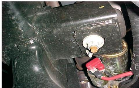
7. IT IS NOT NECESSARY TO REMOVE THE INNER FENDERWELLS, BUT IT MAKES THE INSTALL EASIER ON THE PASSENGER SIDE. TO REMOVE THE FENDERWELLS SIMPLY UNSCREW ALL THE SHEET METAL SCREWS AND FASTENERS ATTACHING IT TO THE FENDER AND FRAME AND THE FENDERWELL WILL DROP OUT.
