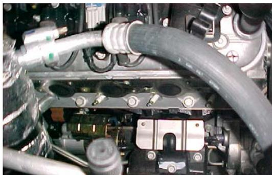
9) INSTALL THE NEW HEADER USING THE SUPPLIED HEAD GASKETS AND BOLTS. TIGHTEN THE GIBSON HEADERS FROM THE MIDDLE BOLTS TO THE OUTSIDE BOLTS. Torque all fasteners to factory specifications.
