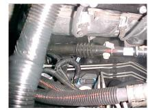
3. On the topside of driver side and passenger side: Disconnect the spark plug wires by grasping and gently twisting the spark plug wire boots. Do not pull on the wires. Set the wires and looms up out of the way. Brush or blow away any debris that may have collected around the manifolds and spark plugs. This will help prevent foreign matter from entering the combustion chambers when the manifolds are removed. Removal of the spark plugs is necessary to avoid accidental spark plug breakage.
