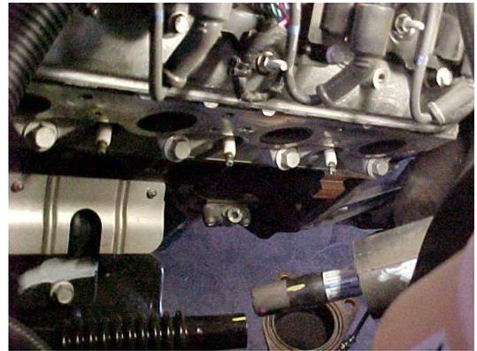
3) **MARK ALIGNMENT OF THE SHAFT BEFORE REMOVING,** THEN REMOVE THE BOLT FROM THE STEERING SHAFT. SLIP STEERING SHAFT APART. NOW UNBOLT THE MANIFOLDS FROM THE STOCK EXHAUST SYSTEM.
