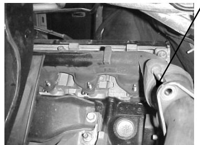
#6 . FACTORY FLANGE CONNECTION. DISCONNECTING POINT.
