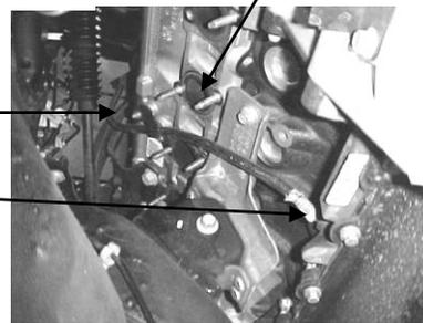
6. THE DIPSTICK MUST NOW BE REMOVED. IT HAS A SEPARATE MOUNTING BOLT ON THE HEAD AND USES AN O-RING SEAL AT THE BOTTOM. USE CARE TO PROTECT THE O-RING. SEE PICTURE #2 ALSO.
