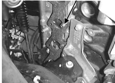
**11.** APPLY A SMALL AMOUNT OF HI-TEMP SEALER TO THE EXHAUST PIPE FLARE THEN INSTALL THE DRIVER SIDE HEADER FROM UNDERNEATH THE VEHICLE. SOME TWISTING AND WIGGLING OF THE HEADER IS NECESSARY. TIGHTEN THE HEADER BOLTS FROM THE CENTER OUT.
