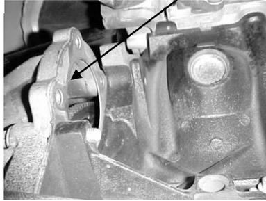
**8.** ON THE PASSENGER SIDE, AGAIN WORKING THROUGH THE WHEELWELL, REMOVE THE NUTS ATTACHING THE MANIFOLD TO THE HEAD THEN REMOVE THE MANIFOLD. REMOVE THE MANIFOLDS ATTACHING STUDS.
