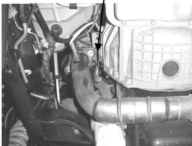
**1A.** DISCONNECT Y-PIPE AT THE FLANGE CONNECTION IN FRONT OF THE CATALYTIC CONVERTER.
