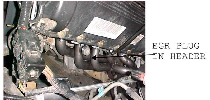
6. THE DIPSTICK MUST NOW BE REMOVED. IT HAS A SEPARATE MOUNTING BOLT ON THE HEAD AND USES AN O-RING SEAL AT THE BOTTOM. USE CARE TO PROTECT THE O-RING. REMOVE STOCK EGR FITTING FROM THE DRIVER'S SIDE MANIFOLD USING WD-40, AND THEN INSTALL INTO HEADER (SHOWN ON PICTURE 2A), USE ANTI-SEIZE ON THE FITTING FOR EASIER INSTALLATION.
