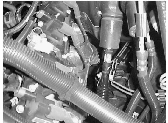
3) **MARK ALIGNMENT OF THE SHAFT BEFORE REMOVING,** THEN REMOVE THE BOLT FROM THE STEERING SHAFT. SLIP STEERING SHAFT APART, BY GRASPING THE UPPER PART OF THE SHAFT (PART ABOVE THE BOLT) AND SLIDING IT UP.
