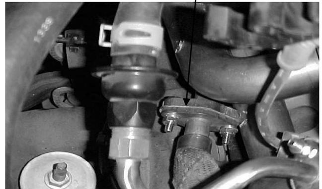
12) FINALLY, MAKE SURE ALL BOLTS ARE TIGHTEN AND EVERYTHING IS RECONNECTED. START THE ENGINE AND LET IT WARM UP. CHECK FOR LEAKS. TURN ENGINE OFF AND MAKE SURE ALL BOLTS ARE TIGHT. **RETORQUE HEADERS AFTER 100-200 MILES.PERIODICALLY CHECK AND RE-TIGHTEN THE HEADER BOLTS. IF YOU DON'T RE-TORQUE YOUR HEADER BOLTS YOU COULD DEVELOP A LEAK AT THE HEAD GASKET. THIS IS NOT COVERED UNDER WARRANTY.**
