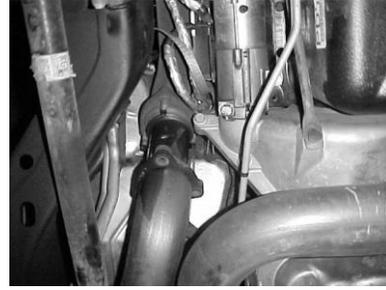
6. Remove O2 sensors cut head pipes. Driver side, cut 11 1/2" forward from weld on front side of converter. Passenger side cut 19 3/4" forward of flange. Use hacksaw or power saw, 18 tooth blade is best, (use eye protection ) file inside so no burs will interfere with new head pipe.
