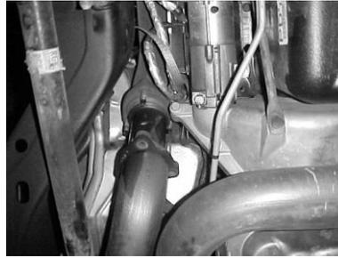
6. Remove O2 sensors cut head pipes. Driver side, cut 11 1/2" forward from weld on front side of converter. Passenger side cut 19 3/4" forward of flange. Use hacksaw or power saw, 18 tooth blade is best, (use eye protection ) file inside so no burs will interfere with new head pipe.
