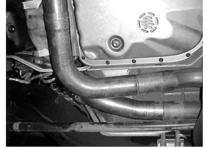
9. On suburbans there is an extra set of coolant lines passing by the headers on the passenger side. Take care to keep these back away from the headers so there is no contact with the tubes.
