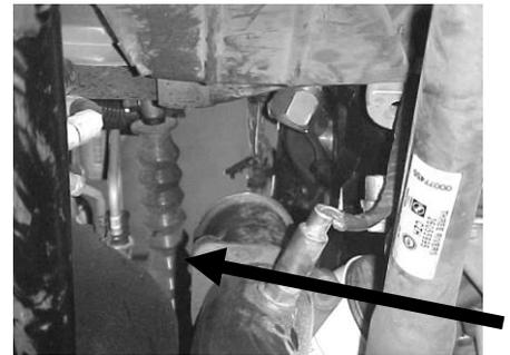
3. On the topside: Disconnect the spark plug wires by grasping and gently twisting the spark plug wire boots. Do not pull on the wires. Set the wires and looms up out of the way. Brush or blow away any debris which may have collected around the manifolds and spark plugs. This will help prevent foreign matter from entering the combustion chambers when the manifolds are removed. Removal of the spark plugs is necessary to avoid accidental spark plug breakage.
