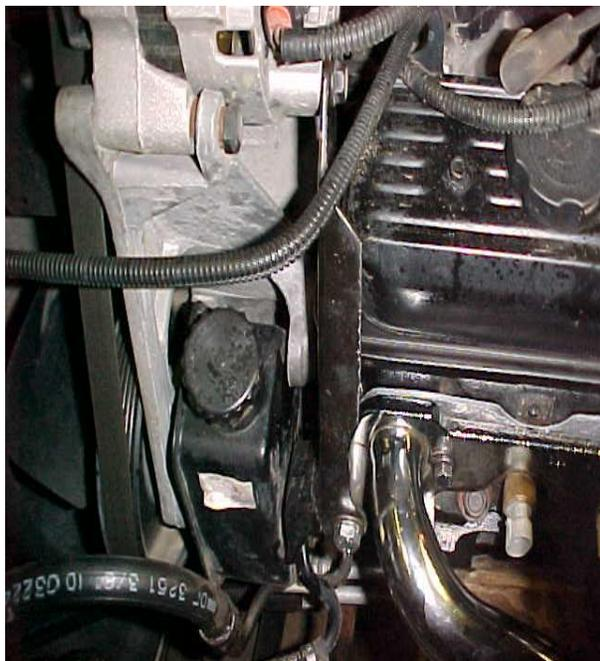
THIS IS A VIEW OF THE MODIFIED BLACK STEEL BRACKET INSTALLED.
