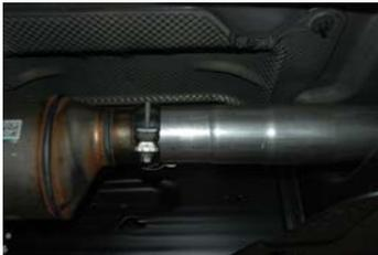
Bolt head pipe #A to the Factory pipe. Insert welded hanger into rubber grommet. Do not tighten.
