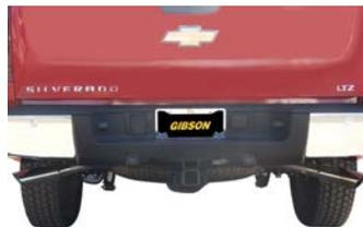
8. Install exit pipes #E onto tailpipes. Cut to your preferred length then use clamps to secure exit pipes to tailpipes. Install stainless steel tips. Clamp down. When you have everything in place, firmly tighten all bolts and clamps down securely. Use stainless steel cleaner weekly to prevent tip from discoloration. Inspect all fasteners after 25-50 miles of operation and re-tighten as necessary.
