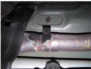
4. Then unbolt head pipe at clamp and remove.
