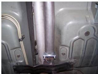
5. Install head pipe #A onto your existing stock front pipe and attach with clamp #F. Use a jack stand to support the converter. Do not tighten.
