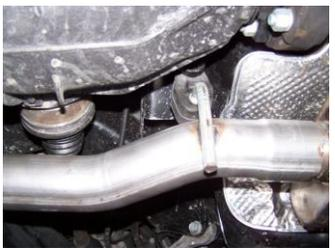
Install driver side tailpipe/muffler assembly #B. Insert all welded hangers into rubber grommets. Secure tailpipes with clamp #D. Do not tighten.
