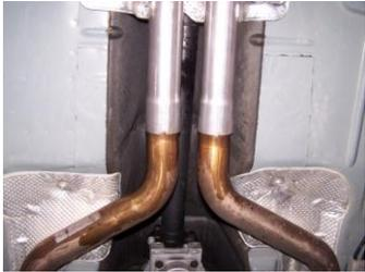
Lay out the exhaust on the floor so it looks like the drawing and compare parts with manual. To remove the stock exhaust, first you must remove the factory cross member under the X-pipe. Then unbolt and remove driver side tailpipe at the flange. Now unbolt and cut tack welds on factory clamps at the X-pipe and carefully remove factory exhaust, save clamps for new exhaust installation. Leave all rubber grommets on hangers. Use WD-40 to help remove hangers.
