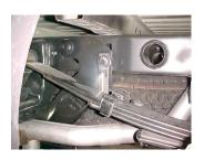
ON PASSENGERSIDE: ATTACH REAR TAILPIPE HANGER #J TO FRAME BY REMOVING THE 18MM HITCH BOLT. THEN RE INSTALL BOLT WITH HANGER
