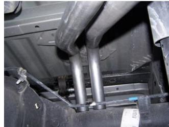
6. Install the driver side over axle tailpipe #C into muffler 1.5-2". Use clamp #H to secure tailpipe and muffler. Insert welded hangers into rubber grommets.
