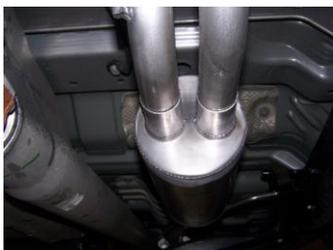
4. Install muffler #B onto headpipe #A 1.5-2" with louvers facing towards the converter. Use a jack stand to support the muffler. Use clamp #G to secure muffler to headpipe. Do not tighten.
