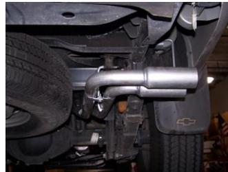
7. Install passenger side tailpipe #D into muffler 1.5-2" and attach with clamp #H. Use bolt kit #I to attach the tailpipes together. Do not tighten. Insert welded hanger into rubber grommet.
