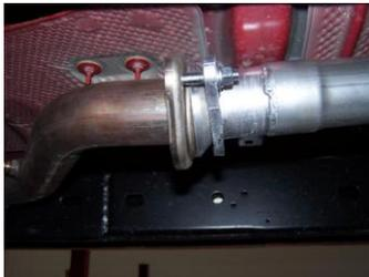
3. Install headpipe #A onto your existing stock 2-bolt flange. Use bolt kit #F to secure. Use jack stand to support converter. Install front muffler hanger #G. Insert hanger into rubber grommet. Do not tighten.
