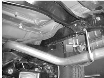
7. Install overaxle tailpipe #C into muffler 1.5"-2". Secure to the muffler using clamp #F. Do not tighten.
