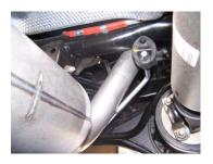
Install the over axle tailpipe #C into the muffler 1-1/2" to 2". Secure to the muffler using clamp #F. DO NOT TIGHTEN. Insert welded hanger into rubber grommet.
