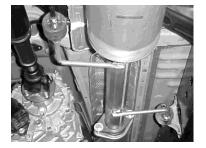
Install head pipe # A on to your existing stock 2 bolt flange. Use hardware kit #G, to secure. DO NOT TIGHTEN. Insert welded hanger into rubber grommet.
