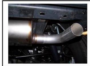
**5b.** Use clamp #E to secure to the exit pipe. Do not tighten.
