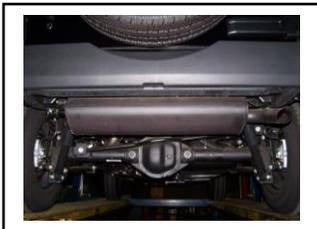
**4.** Install muffer onto head pipe #A 1 1/2"-2" with the louvers facing towards the inlet. Use a jack stand to support the muffer. Use clamp #E to secure the muffer to the headpipe. Do not tighten. Muffer inlet is looking into the louvers.
