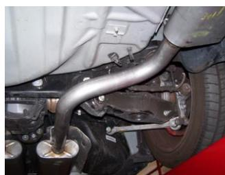
6. Install passenger side tailpipe/muffler assembly #C. Insert all welded hangers into rubber grommets. Secure tailpipe with clamp #D. Do not tighten. Now go back and make sure the first two mufflers in the middle are level.
