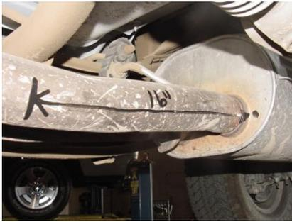
TO REMOVE YOUR STOCK EXHAUST, MEASURE 16" FROM THE MUFFLER FORWARD TOWARDS THE FRONT OF THE VEHICLE. AND CUT THERE LEAVE ALL RUBBER GROMMETS IN PLACE. USE WD-40 TO AID IN THE REMOVAL OF THE EXHAUST AND HANGERS
