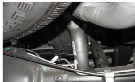
AFTER YOU HAVE CHECKED FOR PROPER CLEARANCES YOU CAN TIGHTEN ALL CLAMPS STARTING FROM THE FRONT AND WORKING YOUR WAY BACK.
