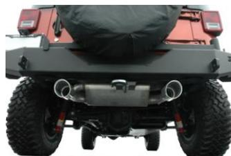
4. Install stainless steel tips. Clamp down. When you have everything in place, firmly tighten all bolts and clamps down securely. Use stainless steel cleaner and a Scotch Brite pad weekly to prevent tip from discoloration. Inspect all fasteners after 25-50 miles of operation and re-tighten as necessary.
