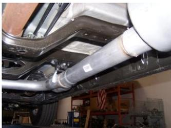
5. Slide resonator #B onto the Y Pipe 1½"-2". Use clamp #G to secure pipes together. Do not tighten.
