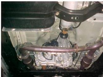
3. Next, unbolt the 2-bolt flanges located just behind the factory converters. Do not discard the factory gaskets and hardware. You will reuse these items when installing the Gibson system.
