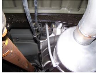
7. Install band clamp #F onto muffler. Insert hanger into rubber grommet. Use provided bolt kit #H. Do not tighten.
