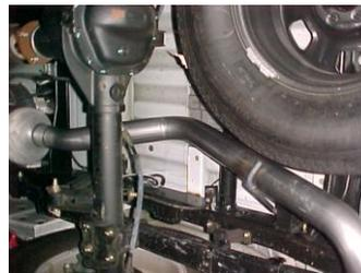
8. Slide over axle tailpipe #D into muffler 1.5-2". Insert welded hanger into rubber grommet. Use clamp #G to secure tailpipe to muffler.
