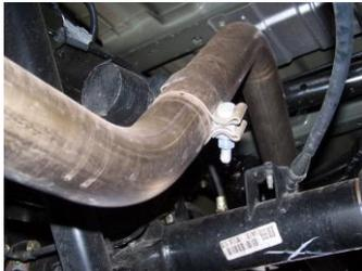
2. To remove your stock tailpipe, remove the clamp shown here. Disengage hanger from rubber grommet. Use WD-40 to aid in this process. Leave all rubber grommets on the factory hangers on the vehicle.
