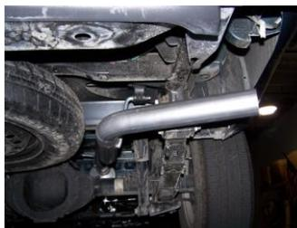
7. Install exit pipe #H onto the tailpipe, use clamp #F to secure the two pipes together. (Rotate for the best fit on your vehicle.)
