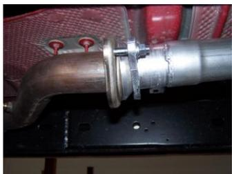
3. Install headpipe #A onto your existing stock 2-bolt flange. Use bolt kit #G to secure. Leave loose until the whole system is installed.
