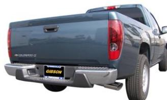
8. Install stainless steel tip. Clamp down. When you have everything in place, firmly tighten all bolts and clamps down securely. Use stainless steel cleaner and a Scotch Brite pad weekly to prevent tip from discoloration. Inspect all fasteners after 25-50 miles of operation and re-tighten as necessary.
