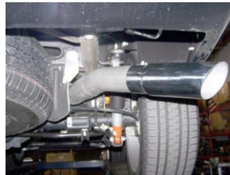
6. Install tailpipe #C into muffler 1½-2" and secure with clamp #F. DO NOT TIGHTEN. Insert welded hanger into rubber grommet.
