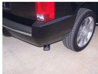
8. Install stainless steel tip. Clamp down. When you have everything in place, firmly tighten all bolts and clamps down securely. Use stainless steel cleaner and a Scotch Brite pad weekly to prevent tip from discoloration. Inspect all fasteners after 25-50 miles of operation and re-tighten as necessary.
