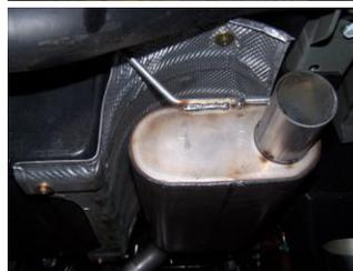
**5.** Install stainless steel tips #D. Clamp down. When you have everything in place, firmly tighten all bolts and clamps down securely. Use stainless steel cleaner and a Scotch Brite pad weekly to prevent tip from discoloration.
