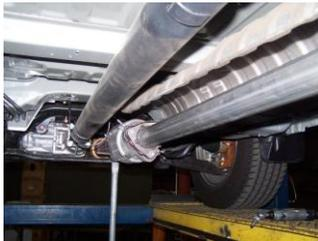
**2.** Bolt head pipe #A onto your existing stock front pipe and attach with factory hardware. DO NOT TIGHTEN. Use a jack stand to support the converter. Insert welded hangers into rubber grommet.
