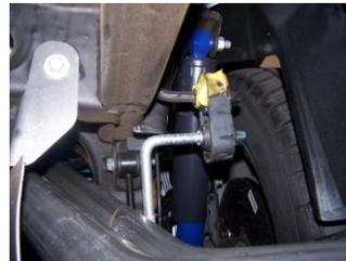
**5.** Install Passenger side tailpipe #D into muffler outlet 1 1/2"-2". Insert welded hangers into rubber grommet. Use clamp #F to attach to tailpipe to muffler. DO NOT TIGHTEN.
