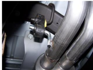
**6.** Install Driver side tailpipe #C into muffler outlet 1 1/2"-2". Insert welded hanger into rubber grommet. Use clamp #F to attach tailpipe to muffler. DO NOT TIGHTEN.
