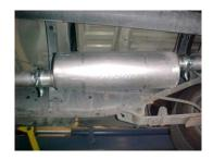
Install muffler #B onto head pipe 1-1/2" to 2" with the louvers facing towards the converter. Use a jack stand to support the muffler. Use clamp #F to secure the muffler to the head pipe. Do not tighten. Muffler inlet is looking into the louvers.
