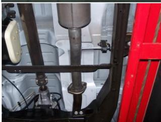
**5.** Install passenger side tailpipe #D to the muffler 1 1/2"-2". Use clamp #G to secure tailpipe to muffler. DO NOT TIGHTEN. Insert welded hangers into rubber grommet.
