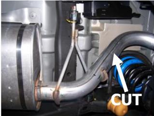
**2.** To remove the stock exhaust, unbolt it from the two bolt flange in front of the muffler. Do not discard you will re-use bolts. Disengage the welded hangers using WD-40 from the OEM rubber grommets. Do not damage or remove the rubber grommets as you will reuse them to mount your new system. Now, cut off tailpipe before and after rear axle for removal.
