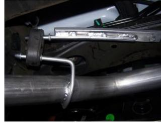
**7.** Install driver side tailpipe #C to the muffler 1 1/2"-2". Use clamp #G to secure tailpipe to muffler. DO NOT TIGHTEN. Insert welded hangers into rubber grommets.
