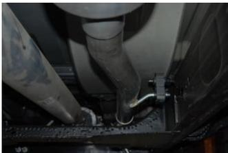
Install muffler #B onto head pipe. Use jack stands to support the muffler. Use clamp #F to secure the muffler to headpipe. Do not tighten.
