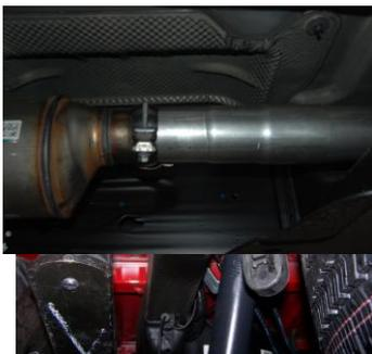
5. Install metal hanger #H into hole located approximately 16" from the rear of the frame. Use hardware kit #I, washer #M, and rubber grommet #J.
