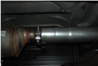
Install adapter pipe #N onto the factory ball mount using the original factory clamp.
