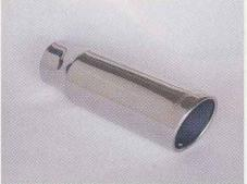
One of the more popular styles of exhaust tips is this Magnaflow angled cut tip. This one is made from polished stainless steel and features a rolled edge.
