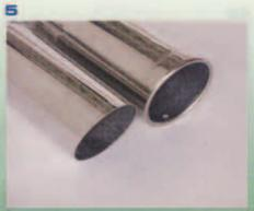
Here you can see the difference between a straight cut tip and one with a rolled edge. The straight cut is more popular but the rolled edge looks more custom. They also are slightly more expansive as well,
