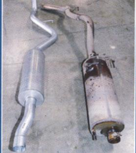
128.13. Shawn then removed the stock exhaust and put it on the floor (pictured next to Gibson's after-cat single exhaust system). This new exhaust includes a 3x21-inch extension headpipe, a superflow muffler, a 3-inch overaxle tailpipe with hangar, a 3-inch exit pipe, a 3-1/2-inch stainless tip, three 3-inch clamps, a band clamp, a band clamp bolt kit, and a front hangar.
