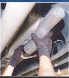
14. Shawn connected the extension headpipe to the OE front pipe, securing it with a 3-inch clamp. Then he inserted a hangar into the rubber grommet and secured it and the rest of the clamps loosely with a 9/16-inch socket and wrench.
