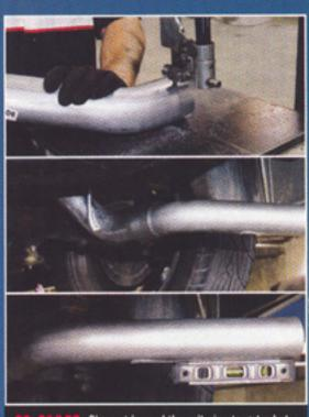
20, 21.822. Shawn trimmed the exit pipe to get a better fit and then attached it to the overade pipe, using a level to determine the best angle.
