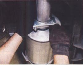
**188-19.** Shawn installed the overaxle tailpipe into the muffler and secured it by inserting the hangar into the rubber grommet. Another 3-inch clamp secured the overaxle pipe to the muffler.
