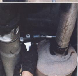
108.11. Shawn removed the clamp just in front of the OE muffler, leaving the stock headpipe and all rubber grommets in place.
