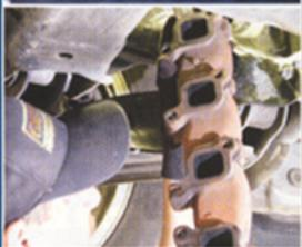
28.3. Being an early bird. Shawn disconnected the Y-pipe assembly from the manifolds before we got there to photograph it: he then removed the starter and set it aside to make way for the removal of the driver-side shock shield and manifold. The OE headers use 10 and 13mm bolts.
