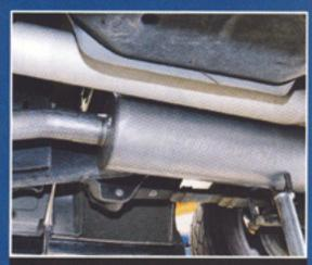
1.8. The muffler installed onto the extension headpipe with the louvers facing the converter. A 3-inch clamp secured the two together.
