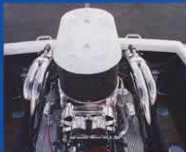
▲ An 8-71 polished huffer from The Blower Shop is bolted to the top of this healthy 468ci Rat motor, and the air and fuel is delivered from a pair of Holley 750s to a complete roller valvetrain. Stainless polished stainless headers show spent gases the door.
