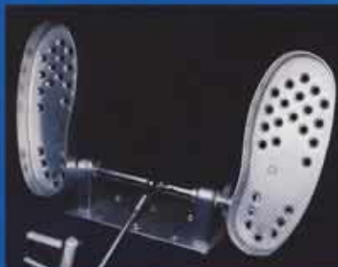
▲ Satin-finished aluminum cavitation plate and throttle pedals allow Bob to adjust the boat's ride and speed with ease.
