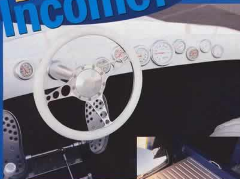
▲ A view of the dash reveals a custom Budnik billet aluminum steering wheel mounted atop a race-style billet steering helm. Gaffrig and Auto Meter white-face gauges supply vital engine information when Bob is stepping hard on the gas.
