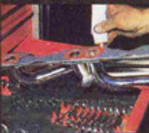
A thin coating of high-temp sealant is applied to both sides of the gasket in preparation of bolting on the new header.
