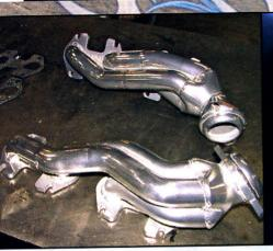
A pair of shorty headers are a popular up-grade with today's late-model, computer controlled engines. These ceramic coated headers are from Gibson Performance. We installed them and the company's cat-back exhaust onto this F-150.
