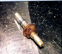
Meticulously, each bolt and stud had to be removed from the engine's cylinder head.
