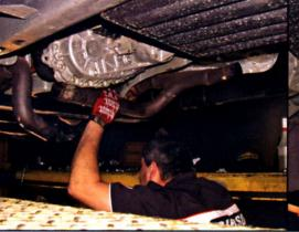
With the transfer case shield out of the way, it was easier for Seidelman to maneuver the Y-pipe to fit together and fit the Gibson system onto the end.
