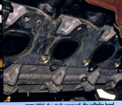
With the studs removed, the cylinder head is exposed and the area needed to be deaned before bolting on a new Gibson gasket and the header.
