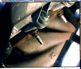
The factory exhaust manifolds work fine, but the airflow can be improved by replacing them with headers. The method to do so is to unbolt and remove the studs.
