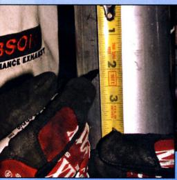
19 Seidelman marks two inches on each pipe to ensure that it slips up to that point. This allows the system to fit together properly.
