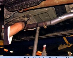
The head pipe is slipped into the rear of the Y-pipe that exits out from the catalytic converters.
