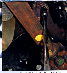
Gibson's R&D technician Shawn Seidelman, began the F-150 installation by unbolting the factory Y-pipe from the manifolds.
