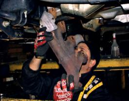
Seidelman, had to remove the truck's 4wd input shaft to remove the driver's side manifold from the vehicle.
