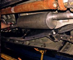
The rear tailpipe section is slipped into the muffler and the system is checked to make sure it all fits together.
