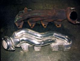
Here's a comparison between the factory exhaust manifold and the Gibson ceramic coated header. The header uses thick flanges and bolts directly to the factory Y-pipe without any modifica-
