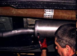
The muffler is slipped onto the head pipe up to the two-inch mark and the rest of the system is assembled in the same manner.
