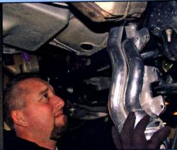
With enough space between the engine and the frame, the Gibson header is maneuvered into the passenger side position.
