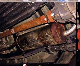
In addition to replacing the exhaust manifolds, we also wanted to replace the restrictive factory exhaust system.
