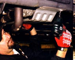
One problem we faced in trying to reconnect the factory Y-pipe was that there wasn't enough room to maneuver it. Seidelman had to temporarily remove the transmission transfer case shield.
