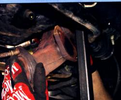
Removing the passenger side manifold was a bit more difficult. Seidelman had to move the starter aside and lift the engine a couple of inches before gaining enough room to remove the manifold.
