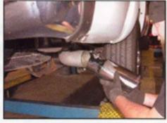
Install stainless steel tip. Clamp down. When you have everything in place, firmly tighten all bolts and clamp down securely. To clean stainless steel tips use any stainless steel cleaner and scotch brite pad.
