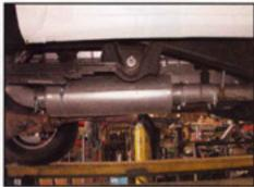
Install band clamp H with welded hanger onto muffler. Insert welded hanger into rubber grommet. Tighten band clamp using hardware I. Install the turnout pipe D on to the tailpipe. Secure together with clamp G. Do not tighten. Roll the exit pipe until it is at the correct angle for your truck. Insert welded hanger into grommet.
