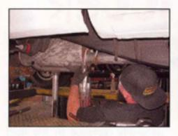
To remove your stock exhaust, cut off your stock system just in front of the muffler after the weld, and leave all rubber grommets on the hangers. Use WD-40 to aid in the removal of exhaust and hangers.
