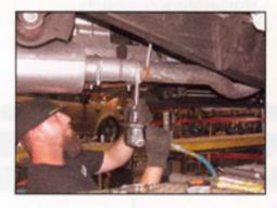
Install head pipe A on to your existing stock front pipe and secure with clamp F. Do not tighten. Install muffler onto head pipe A 1-1/2" to 2" with the louvers facing towards the converter. Use a jack stand to support the muffler. Use clamp G to secure the muffler to the head pipe. Do not tighten. Muffler inlet is looking into the louvers.
