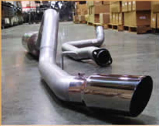
Large 4 -inch mandrel-bent tubing.
