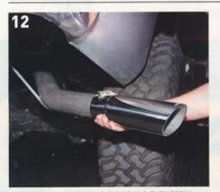
FINALLY, SLIP ON THE STAINLESS TIP AND THEN BEGIN TIGHTENING THE ENTIRE EXHAUST SYSTEM, WORKING YOUR WAY FROM THE FRONT TO THE BACK.
