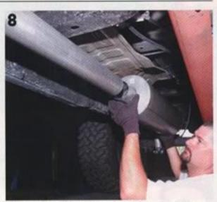
THE RESONATOR AND THE SUPERFLOW MUFFLER WILL BOTH SLIDE INTO PLACE AFTER THE Y-PIPE.
