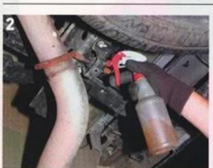
A FEW SQUIRTS OF WD-40 WILL ENSURE THAT THE HANGERS FOR THE TAILPIPE AND MUFFLER SLIDE OUT OF THE RUBBER GROMMETS EASILY.
