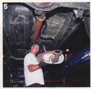
ONCE THE Y-PIPE IS DISCONNECTED, IT CAN BE COM-PLETELY REMOVED FROM BENEATH THE TRUCK.
