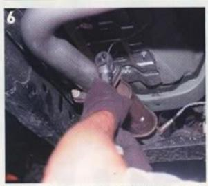
THE NEW GIBSON Y-PIPE WILL LINE UP WITH THE FLANGES ON BOTH SIDES. BOLT THE PIPE ON AND DON'T FORGET TO RECONNECT THE GROUND ON THE DRIVER SIDE.
