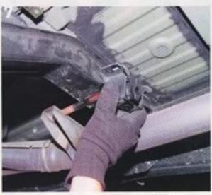
SLIDE THE RUBBER GROMMET ONTO THE GIBSON HANGER AND BOLT IT BACK TO THE FRAME.
