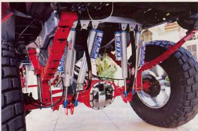
All of the chassis has been either chrome-plated or powdercoated red, including the DR The Edge suspension system and tricked out axle housings. Check out the shock mounts fabricated to house four of the eight King bypass tube shocks.
