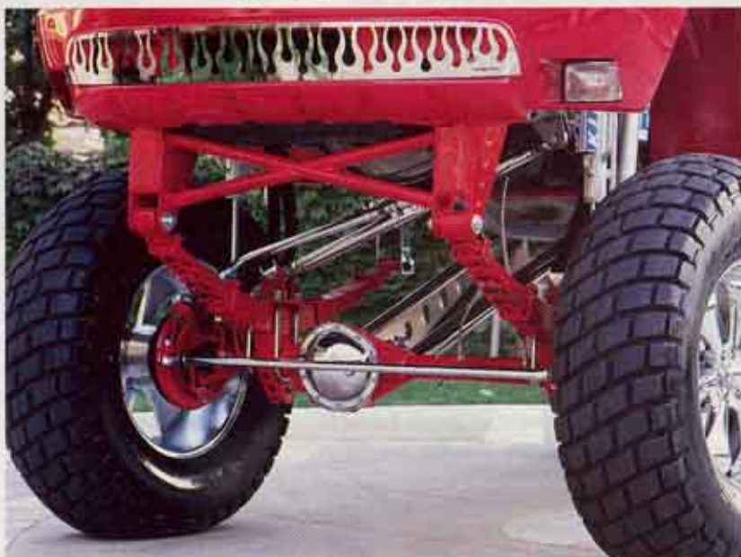
What began as a two-by front suspension has evolved into a larger-than life four-by setup consisting of a Donahoe Racing 10-inch leaf spring lift kit, strengthened hangers and a built axle featuring ORU crossover and hydraulic steering.
