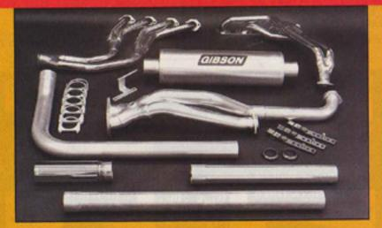
Some of Gibson's most popular items are its power exhaust systems, designed to give a motorhome increased climbing and passing power. They're 50-state emission legal and are aluminized and mandrel-bent to last long and stay strong. The exhaust systems also feature:
