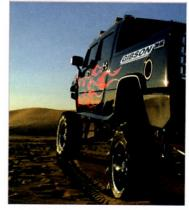
sparks stopped raining, the H2 had a whole new profile. A five and a half foot long truck bed was added to the back. To do this, Ultra Limos had to add twenty inches in front of the rear axle and fourteen inches behind the rear axle to evenly distribute the weight and the trucks new center of gravity. What was next on the list?
