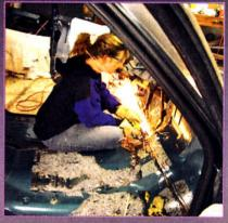
Here is the photo to prove that Bobbie doesn't just own but also had a part in the build of the truck. She is cutting the floor of the cab for the body-dropping action.
