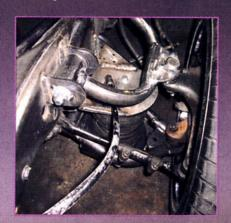
As you can see, this is a full custom, and that also goes for the suspension. Shown here are the custom-made control arms for the front end.
